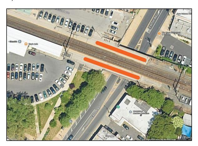
Due to concerns that the work on the topside of the bridge deck could generate construction debris below the bridge, flagging a single lane of traffic is required as a safety precaution.
